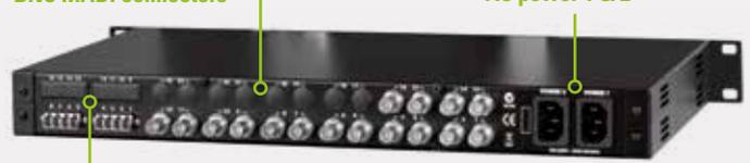
Up to 16 LC connectors for WDM or CWDM multiplexers and external fiber protocols
